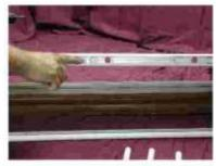
Insert Mounting Bracket into first Horizontal Bar on Both sides.
